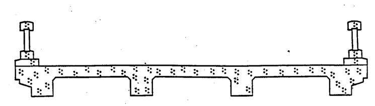
ROADWAY CROSS SECTION CONCRETE DECK GIRDER
