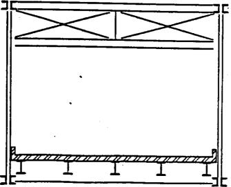
THROUGH TRUSS (ITEM 43, BRIDGE TYPE = 310 FOR SIMPLE TRUSS SPAN ILLUSTRATED.)
