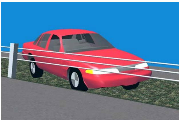
FIGURE 5 Underride potential of single-cable engagement
