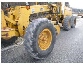
(14) Blading 2" Aggregate with Motograder
