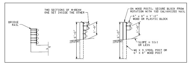
Figure 16 - Guardrail Height Detail
