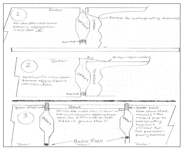
Figure 9 - Grouting Details for Beams with Differential Camber
