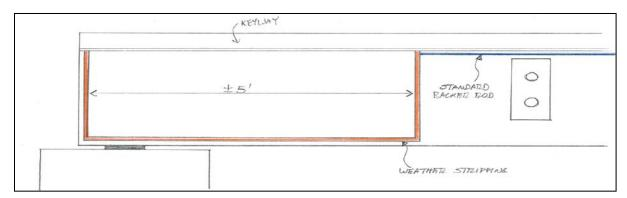
Figure 7 - Full Depth Grouting Procedure to Prevent Beam Rollup
