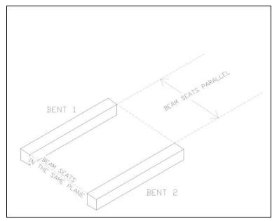
Figure 1 - Dunnage Alignment at Beam Seats
