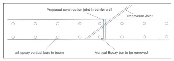
Figure 12 - Rebar Cut on Skewed Beam
