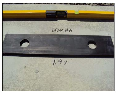
Figure 4 - Documenting Slope of Beam Seat with Smart Level
