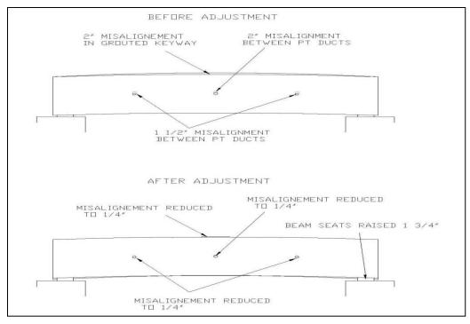
Figure 6 - Adjusting Beams to Align Post Tensioning Ducts
