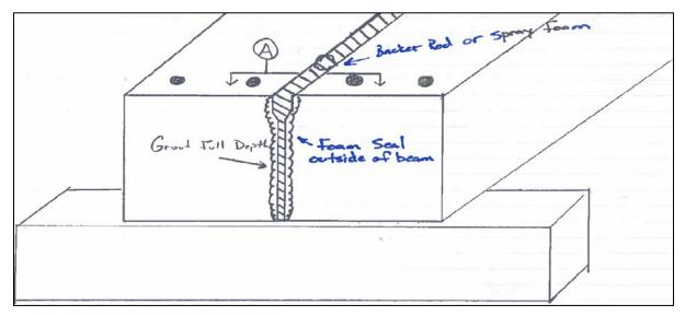
Figure 8 - Backer Rod or Spray Foam Used as a Seal Against Leakage
