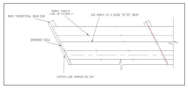
Figure 5 - Markings for Beam Layout
