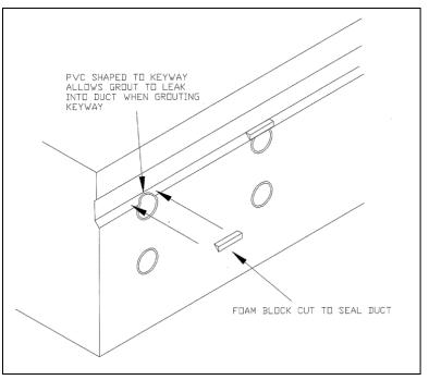
Figure 2 - Half Keyway Glued Above Conflicting Duct
