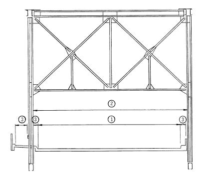
Item 51 - Bridge Roadway Width, Curb-to-Curb Item 52 - Deck Width, Out-to-Out Item 50 - Curb or Sidewalk Width (1) (2) (3)
