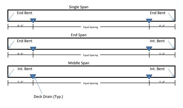
\*\*Note: Equal Spacings were rounded to the nearest inch. A 12" clear gap in reinforcement shall maintained within 12" of the drain locations.
