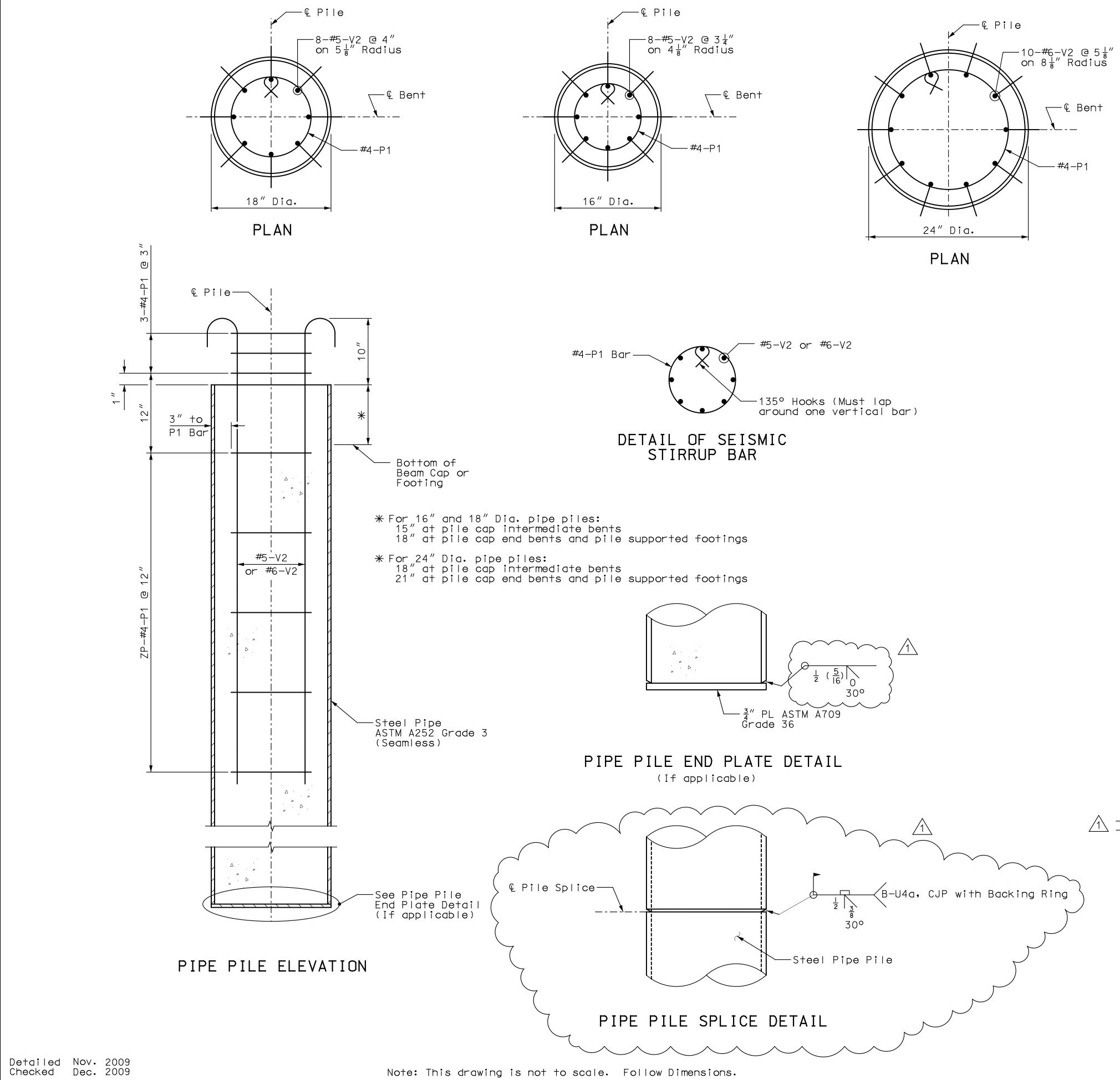
Notes: All concrete for steel pipe piles shall be Class B-1.
