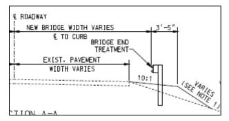
Figure 15 - Shoulder Slope Detail
