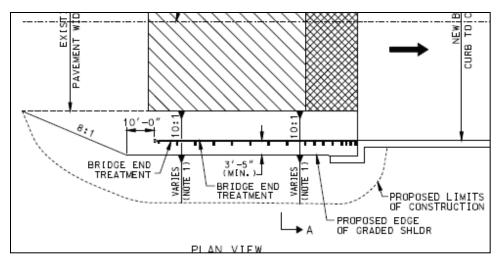
Figure 14 - Shoulder Widening Detail
