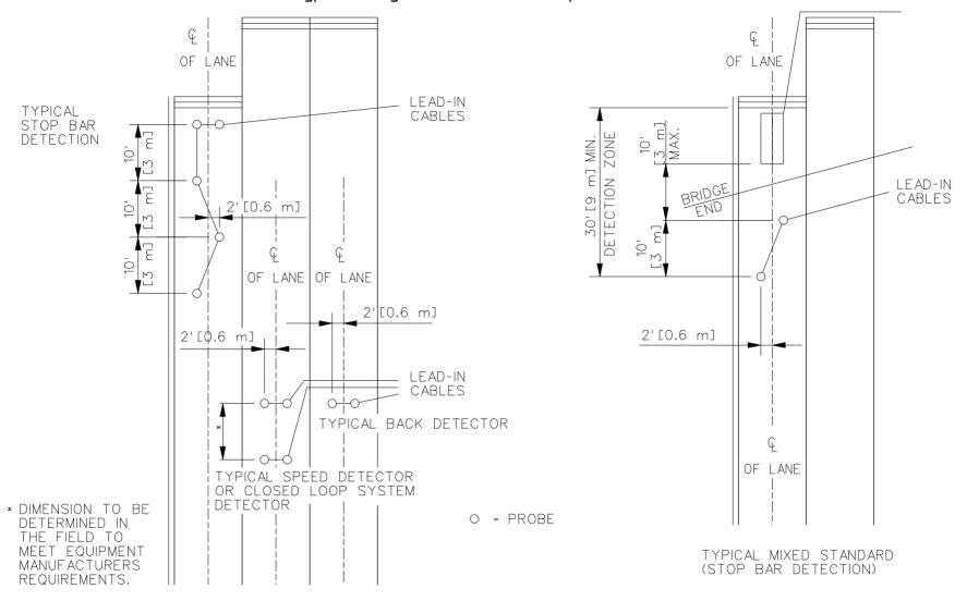
NOTE: IF POSSIBLE, AVOID INSTALLING PROBES OVER TRAFFIC ON OVERPASS BRIDGES.
