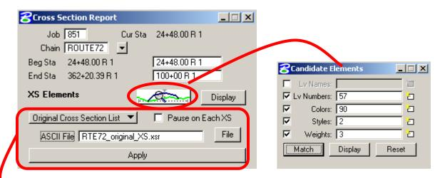
Choose **Original Cross Section List** from the pull down. You can choose to **Pause on Each XS**. Type in the name of the ASCII file with the extension of .xsr. This file will be placed in the working directory.
