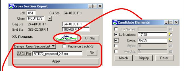
Choose **Design Cross Section List** from the pull down. You can choose to **Pause on Each XS**. Type in the name of the ASCII file with the extension of .xsr. This file will be placed in the working directory.
