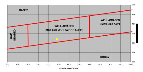
When the point is located in the area entitled, "Well-Graded (Max Size 2", 1 ½", 1" & ¾")," the combined aggregate gradation is considered suitable for use in an optimized concrete mix. When the point is located outside this area, the mix needs to be evaluated by the Materials Field Office.
