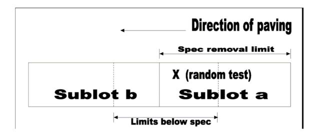
In this example the random QC sample fell late in sublot a and test results indicated that voids were below the limits for removal. By specification sublot a should be removed.
