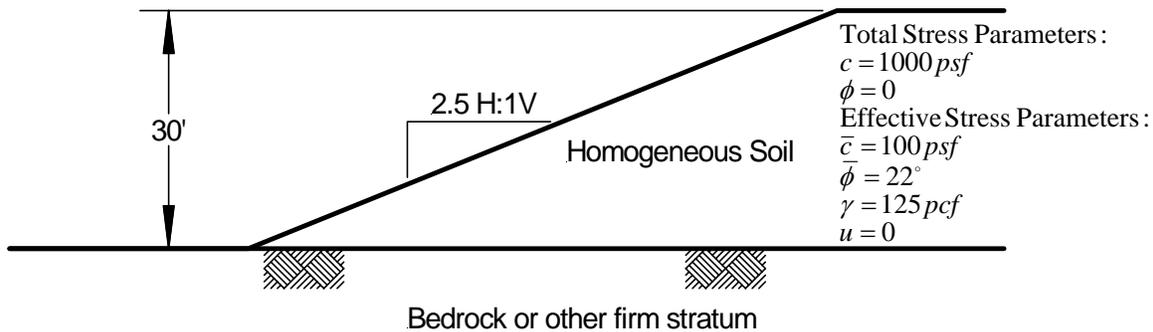
Figure 4.1 Slope conditions used for example problem.
