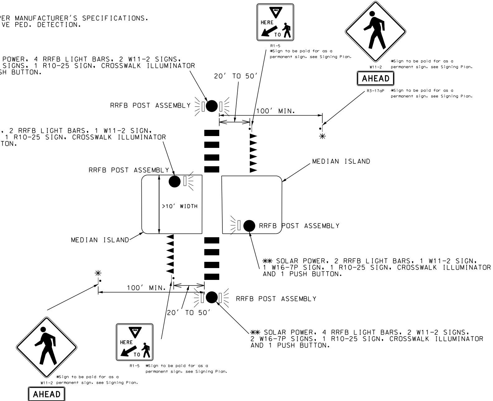
\* ACTUAL ADVANCED SIGN LOCATION WILL BE BASED ON FIELD CONDITIONS AND DETERMINED BY THE ENGINEER.
