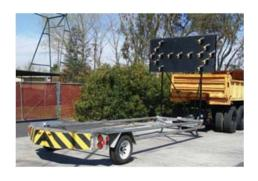
operate Vorteq TL-3 Trailer TMA is lightweight and attaches to most host vehicles with a 20 ton pintle hook and 7 pin electrical connector. Acceptable host vehicle weight is 9960 lbs. to infinite weight. Super fast attachment means you have full TMA protection in less than a minute. The open frame design means inspection and maintenance is quick & easy.
