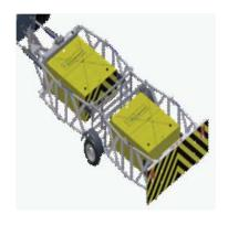
The SST TMA meets all standard and optional NCHRP 350/MASH TL-3 test requirements to provide optimum protection to drivers, equipment, and the public.
