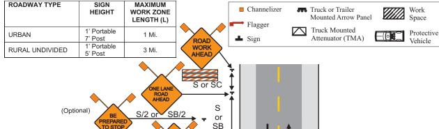
A protective vehicle **may** be used while work is in progress. The protective vehicle **may** be equipped with a TMA and/or flashing arrow panel and positioned at least 150 ft. in advance of the work space.
