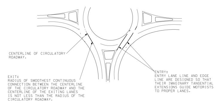
Vehicle Path Overlap at Two-Lane Roundabouts. Figure 11
