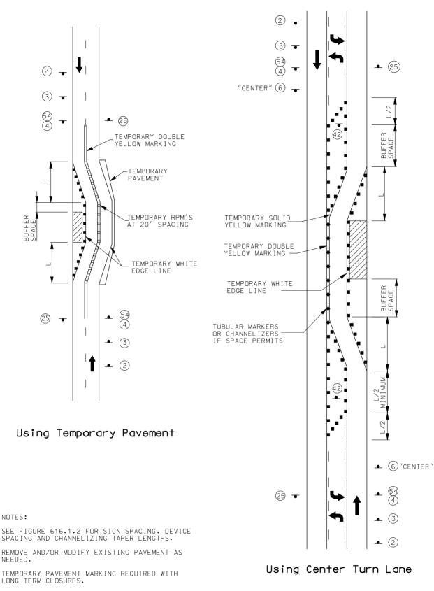
FOR SHORT TERM OPERATIONS WHERE IT IS NOT FEASIBLE TO MODIFY PAVEMENT MARKING. DEVICE SPACINGS ARE ONE-HALF OF THE SPACING SHOWN ON FIGURE 616.1.2.
