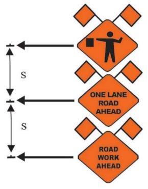
The advance warning area contains warning signs with appropriate legends, regulatory signs, such as speed reduction signing, changeable message signs and other warning devices. The signs or other warning devices are positioned to give the driver sufficient time to react to the conditions. Warning devices are not to be placed too far in advance, as the warning message will lose effectiveness. Suggested advance sign spacing information is shown below.
