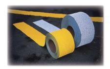
retroreflectorized tape with a pressure-sensitive adhesive on the back. The tape, available in white and yellow, may be used to provide a surrogate permanent pavement marking or it may be cut into 4-ft. long sections and applied to the road surface at 40-ft. intervals as a temporary pavement marking. The length and spacing of the latter pavement marking may be reduced to one-half when
