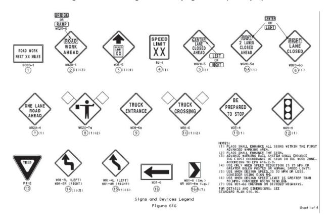
Using the example above the first set of advanced warning signs shall be flagged. Additional flagging requirements can be found in the device legend.
