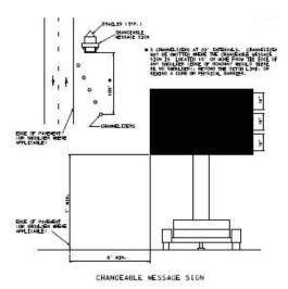
be positioned on the upstream end of the unit to form a taper leading up to traffic side of the unit. The recommended length of this taper is 100 ft. For a sign located in the median, the sign should be delineated from both directions.
