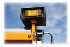
equipment while in the temporary traffic control zone. All work vehicles and equipment shall be equipped with an acceptable warning light system. These lights shall be activated whenever a vehicle or piece of equipment is engaged in a work zone or incident response operation within the temporary traffic control zone. An exception to this requirement is those vehicles and pieces of equipment located within a workspace delineated by channelizers or protected by
