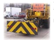
traffic control signs affixed to a protective vehicle or pilot car at a **recommended minimum height of (4) four feet (48 inches),** measured vertically from the bottom of the sign to the pavement surface.
