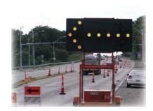
capable of flashing displays. The devices are intended to provide additional warning and directional information to assist in traffic movement through or around a temporary traffic control zone. These units may be either trailer- or truck-mounted. However, truck-mounted units are preferred in mobile operations.
