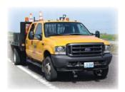
Protective vehicles are used to safeguard the workspace from errant vehicles. In some operations, these devices also serve as platforms for signs and other devices used to warn traffic of upcoming conditions or inform them of needed actions. For increased motorist, driver and worker safety, the protective vehicle may be equipped with a truck-mounted attenuator.
