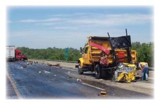
Due to the placement of temporary traffic control devices in relation to traffic, these devices shall be crashworthy. This requires that all temporary traffic control devices conform to the crash test requirements of the National Cooperative Highway Research Program (NCHRP) Report 350. Exceptions to this crashworthiness rule are those state-owned devices that have received grandfather status (e.g. pre-10/98
