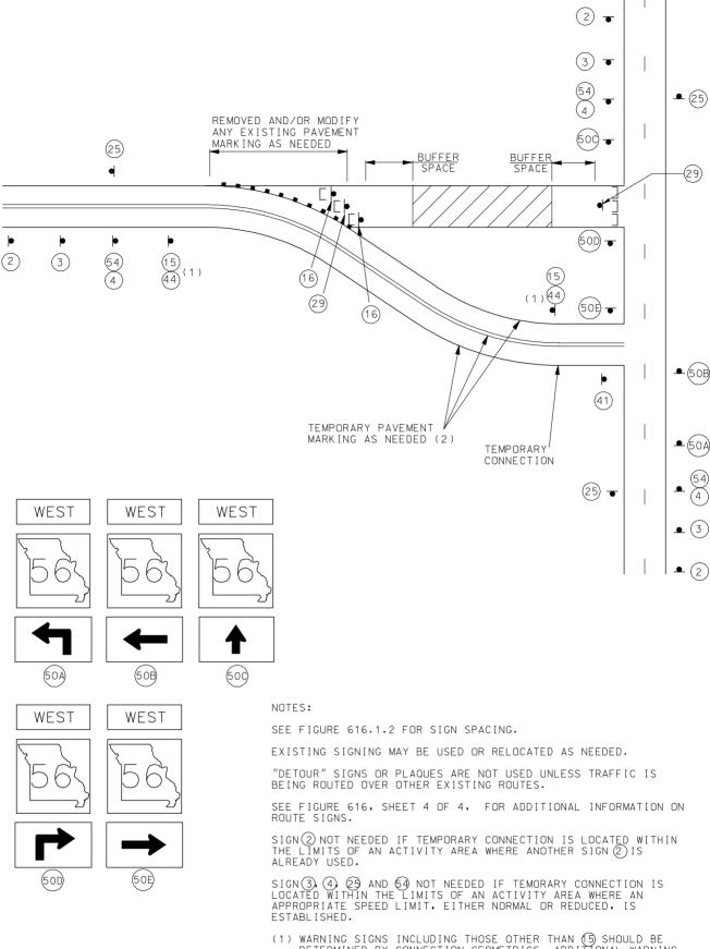
(1) WARNING SIGNS INCLUDING THOSE OTHER THAN (5) SHOULD BE DETERMINED BY CONNECTION GEOMETRICS. ADDITIONAL WARNING SIGNS MAY ALSO BE NEEDED.
