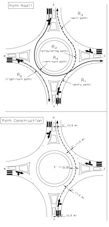
FOR EACH LEG OF THE ROUNDABOUT, THE 5 PATH RADII ILLUSTRATED AT LEFT ARE MEASURED. THE RADII ARE MEASURED BY CONSTRUCTING PATHS AS SHOWN BELOW LEFT. THE ASSUMED VEHICLE CENTERLINE IS OFFSET 5' (1.5 m) FROM CURB FACE, 5' (1.5 m) FROM ROADWAY CENTERLINES, AND 3' (0.9 m) FROM A PAINTED EDGE LINE.
