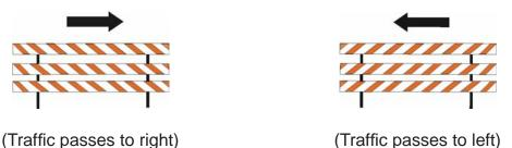
• Where both right and left movements are provided, the stripes should slope downward at a 45 degree angle away from the center of the barricade array.
