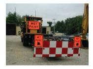
Truck-mounted attenuators are energy-absorbing devices attached to the rear of trucks used as protective vehicles. These devices are designed to protect the motorist and protective vehicle driver upon impact.
