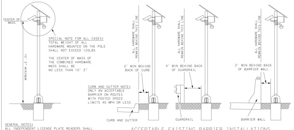
BE LOCATED BEHIND EXISTING BARRIER AS DEPICTED ON THIS SHEET AND THE INSTALLATION SHALL BE A MINIMUM OF 50 FEET FROM THE END OF THE BARRIER. GUARD CABLE IS NOT DEPICTED AS AN OPTION DUE TO ITS 12 FOOT DEFLECTION DISTANCE.
