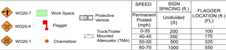
Use this supporting figure when the work space is more than 500 feet and less than 3 times sign spacing from the nearest intersection.
